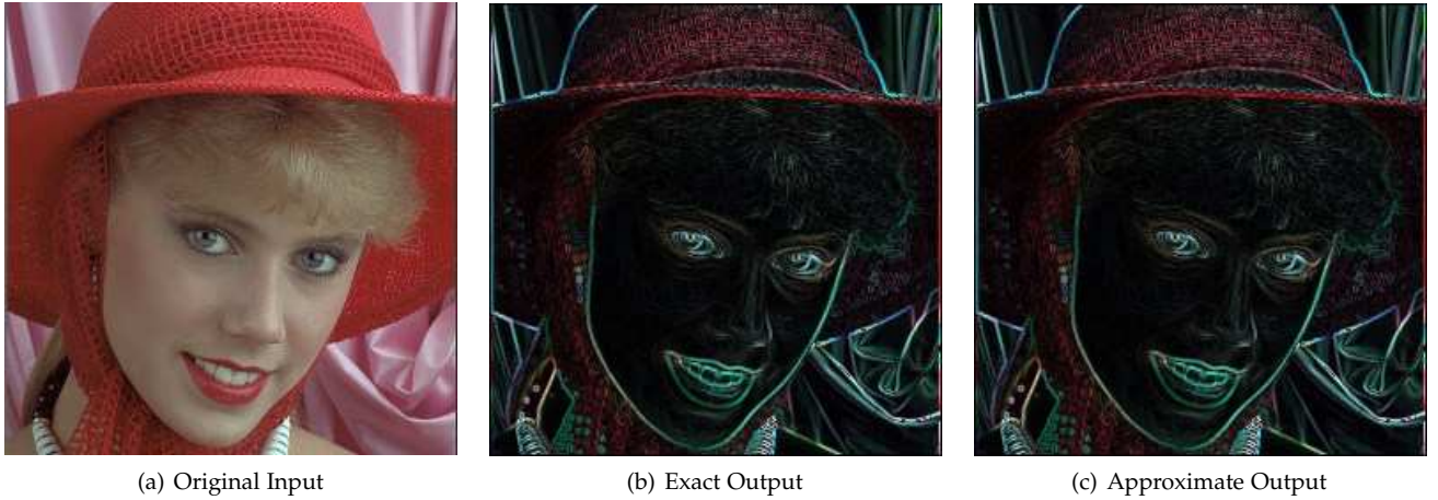
Fig. 4: (a) Original input image. (b) Error-free exact Sobel filter output with PSNR = inf. (c) Error-injected approximate Sobel filter with PSNR = 30dB.
